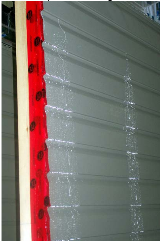
Figure 6 Example of face drainage from drain holes in vinyl siding (Profile #2)
