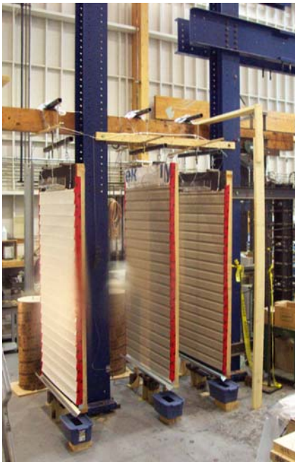
Figure 2 Overview of test set-up for weighing test walls during drainage/drying testing.
